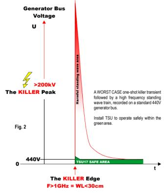
Correspondingly, it appears that life expectancy can be attributed to individual engineers working methods. One engineer may instantly disconnect a generator under load, while other correctly offload the generator before disconnection.
