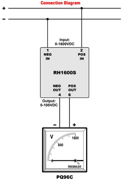
Input: 0-100VDC Scale: 0-1600VDC
