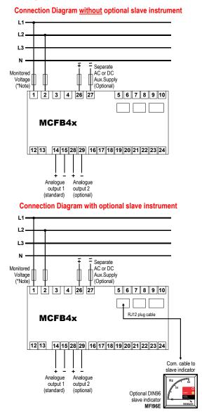
\*Note: The standard models takes the auxiliary supply voltage from the monitored voltage (terminal 1 & 2).
