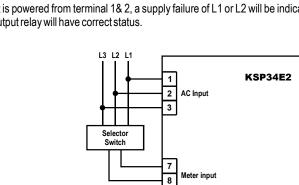
Relay shown de-energised, and energises only when phase sequence is correct and supply condition is normal.
