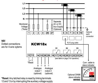
NB! To ensure correct kW measurement, the voltage phase sequence
