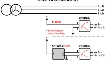
The instrument will detect earth fault on all phases independent of which phase is connected to terminal 4.
