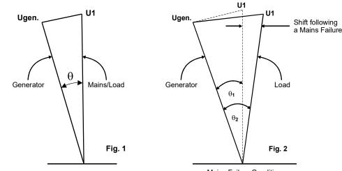
Mains Failure Condition
