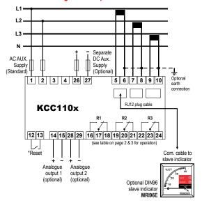
\*Reset Any latched relay is reset by linking terminals 12 and 13 or by interrupting the auxiliary voltage supply.
