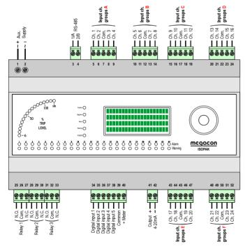
: Operates when the danger limit of a channel is exceeded
